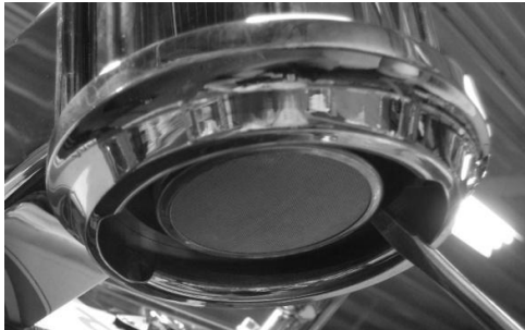
Figure 9a (left). Pry left and right with screwdriver to remove group screen and rubber group seal.
