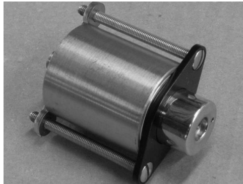
Figure 24. Progressive pre-infusion cylinder isolated from machine, the mounting parts that hold the cylinder to the machine are also shown. (In fact, the retaining ring that holds the upper end of the cap is not mounted, for that reason, the piston end is not flush with the outside)
