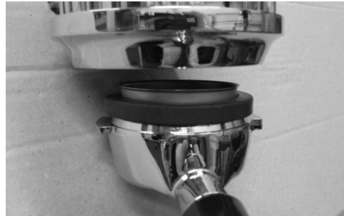
Figure 9a (left). Pry left and right with screwdriver to remove group screen and rubber group seal.
