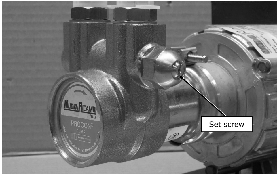
Figure 7. Showing the set screw on the pump to change pump pressure.
