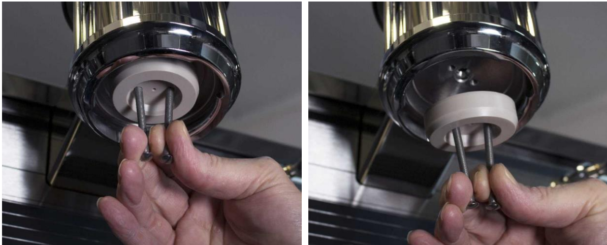
Figure 18. How to remove the dispersion base if it does not come out easily. Use 2 bolts M5x60 or similar to get grip onto the dispersion base.
