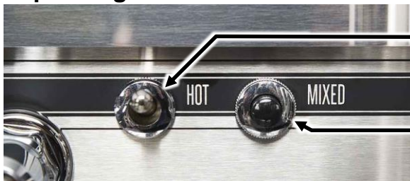
Figure 9. The hot-water toggle switch and mix-water push button switch.
