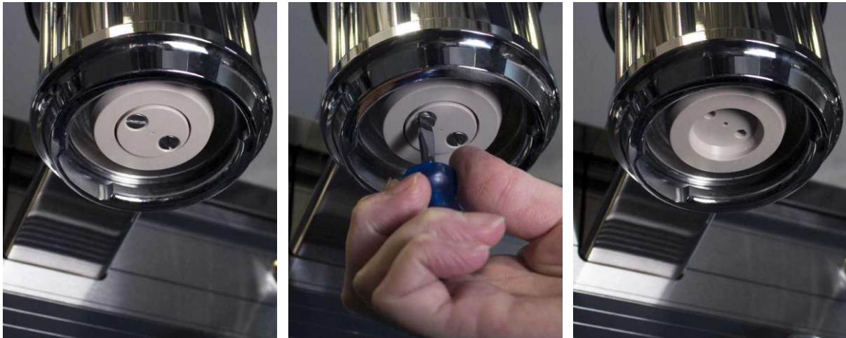
Figure 17. Dispersion set mounted in group head. Remove the 2 screws. The dispersion plate will fall out. The dispersion base remains in the group.
