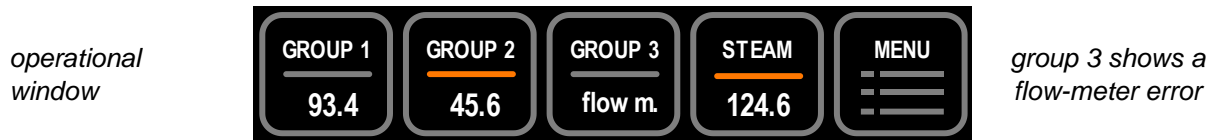
Figure 20. Error report if the flow-rate during a brew falls outside the flow-meter range.
