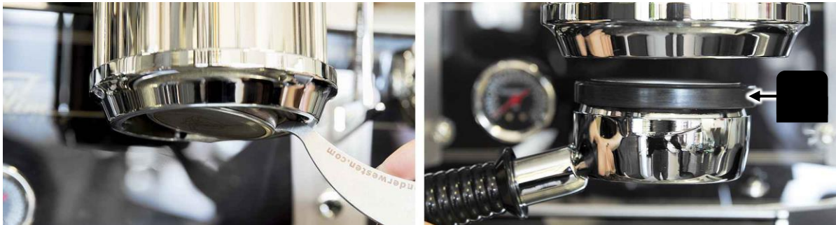
Figure 16 a (left). Pry left and right with screen extractor to remove group screen and group seal.
