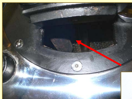
The heating element inside the drum with its heat shield
