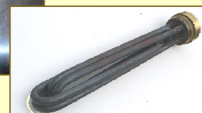
The heating element inside the drum with its heat shield
