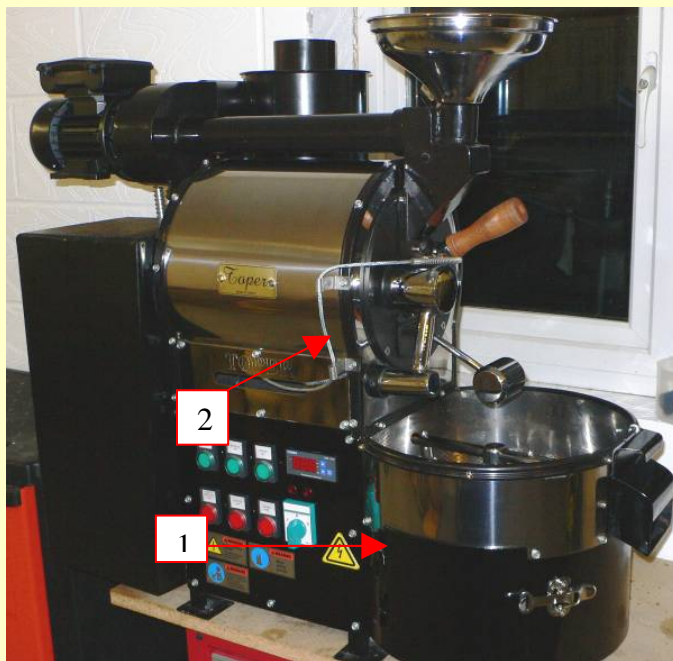
Side View & Rear View, Cooling tray chaff removal hatch (1), Thermocouple lead (2), Industrial Motor driving roaster airflow (3), Housing covering impeller fan and top tube drawing air/chaff from roasting chamber, Control Panel (5), Cover for industrial motor and chain drive for drum (6).
